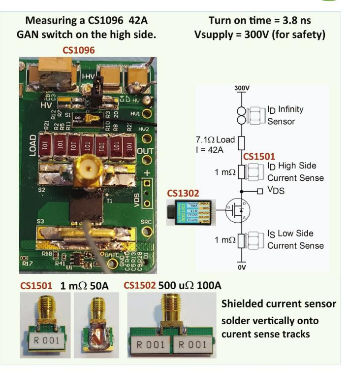
The sensors are based on Ohmite FCSL110 1mOhm metal foil resistors, which are 11mm wide x 5mm high. The active surface is downwards to minimize inductance. The CS1501 sensor is rated at 50 A, with a maximum inrush current of 240A, and the CS1502 is rated at 100A.
