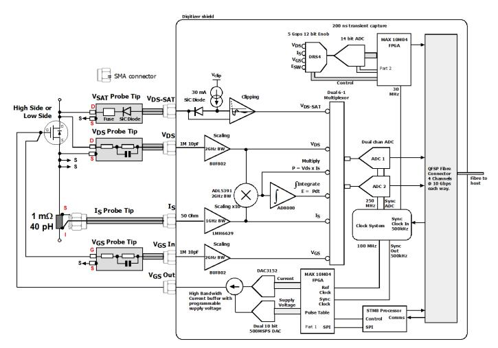
We are introducing a two channel ADC, so we can measure any two parameters at the same time. The 5GSPS DRS4 digitizes  $V_{DS}$ ,  $I_{S}$ ,  $V_{GS}$  and  $E_{SW}$  all at the same time, and all are returned to the CS548.
