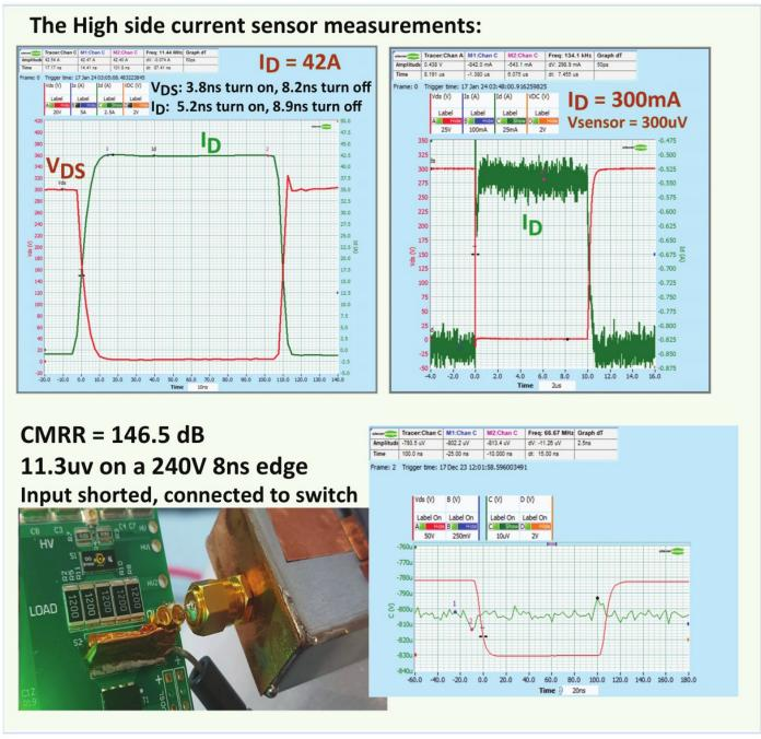
We want to achieve 1 part in 1000 for reading the current, or 50mA on 50A. The 300 mA capture graph shows the current could have been at 50 mA (50uV at the sensor), and can still be resolved. The next version of the current sensor will be a bit quieter, as we learnt some lessons.
