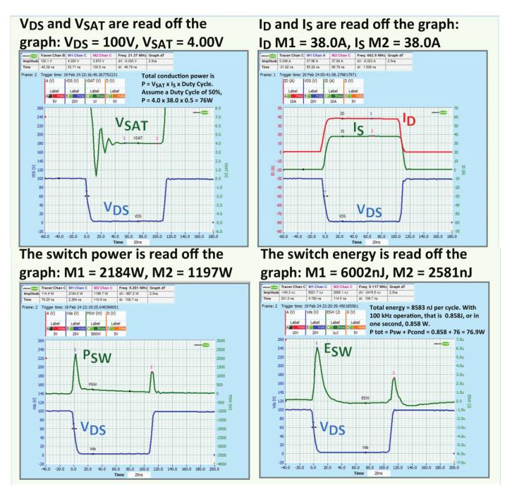
Note that the measured pulse is about 100ns wide. Vsat is oscillatory while the reverse diode capacitive charge dissipates.
