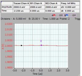
With a 1.28us moving average the amplitude of the noise in the tracking graph has reduced to the sub mv level.
