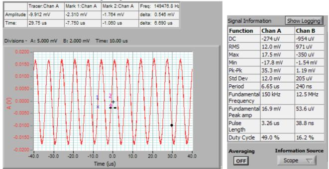
The Std Dev is 12 mV. (Note the Fundamental peak amp is given in peak units, which are  $\sqrt{2}$  times higher than the RMS value). The frequency graph shows:
