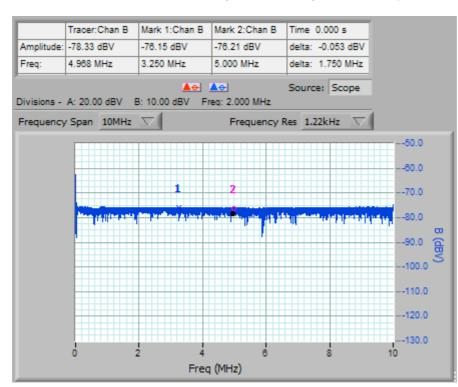
We can see that the cross talk is not frequency dependant, and is a fixed –76dB. This is equivalent to 1 part in 6300. Thus we achieve better than 12 bit performance, provided the interferer is of less amplitude than the peak signal expected on the signal of interest.
