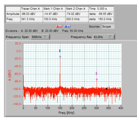
As the gain drops (the FSD has changed from 200mV to 800 mV), the noise floor has increased. This is because at high gains the noise floor is limited by the front end amplifier noise, while at lower gains we see a transition to the intermediate gain chain output noise dominating the noise floor.
