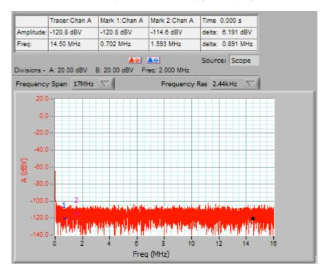
This shows fairly clearly that the noise is externally sourced. It also tells us that even short stubs of wire or PCB track can act as antennas for signals we did not expect. To maximize dynamic range for low level signals you will need good shielding around all the circuit modules used – particularly when used near PC's and LCD display's.
