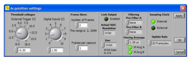
The Moving Average time constant sets the sample time period that is averaged to achieve one output sample. In the example above this is 1.28 us (128 samples at 10ns/sample). The average takes the last 128 samples, averages them, and emits the new value. On the next sample being received, a new average is calculated again, based on the last 128 samples (one of which will be new). We use internal buffers to ensure that the averaged, non-averaged and digital values all remain synchronized.
