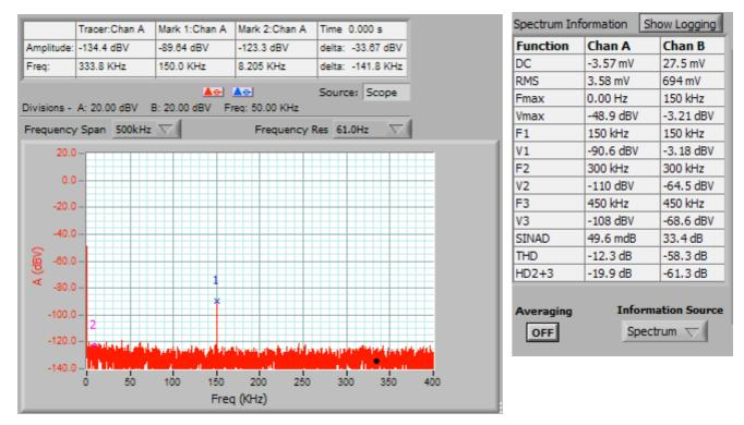
After averaging 20x, we have improved the noise floor to about -120 dB. The dynamic range has increased by about 20 dB (or 10x, about the same as an extra 3 bits of resolution).
