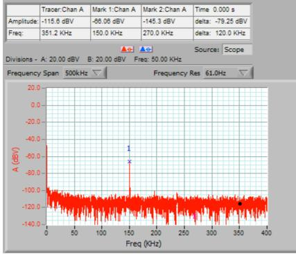
The noise floor is about 20 dB lower with averaging. Increasing the number of averages can make further gains.
