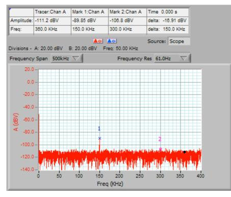
We have a noise floor now of about -105 dBV, so a margin of 15 dB on the -90 dBV signal.
