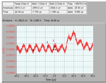
The 200 uV jump in level between 10 and 20us is caused by the trigger LED coming on, and injecting charge into the analog front end. We have filtering to try and minimize this effect. This problem has since been resolved.
