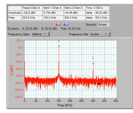
As can be seen the signal generator output noise is now dominating. We see a noise floor of about –80 dBV, giving a dynamic range of about 84 dB. This is marginal for 14 bit measurements.
