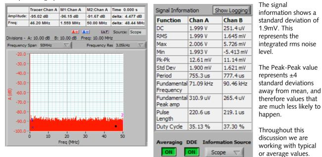
We have a dynamic range of  $\pm 2500$  mV, with a standard deviation of 1.9mV. This is 1 part in 2630. The SNR =  $20 \log(2500/1.9) = 68.4 \text{ dB. ENOB} = (68.4-1.76)/6.02 = 11.1 \text{ bits ENOB}$ . This is the basic capability of the scope.
