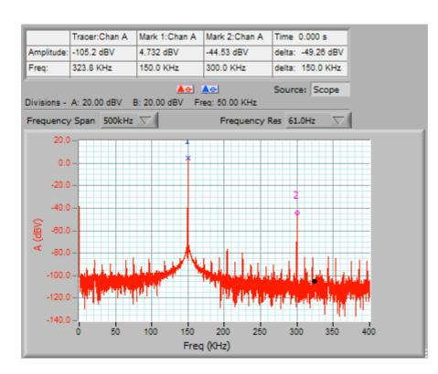
The features seen are probably remnants of the internal signal generator power supply, and digital processing system. We removed the input signal, while continuing to sync off the channel B sync signal. The result is below:
