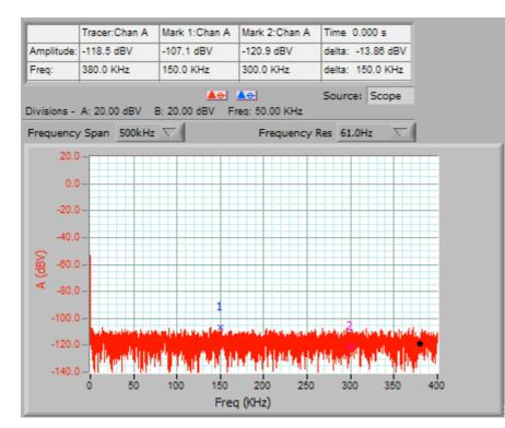
This is the averaged response with no input signal, with 5V FSD input range, as used to measure the spectra above.
