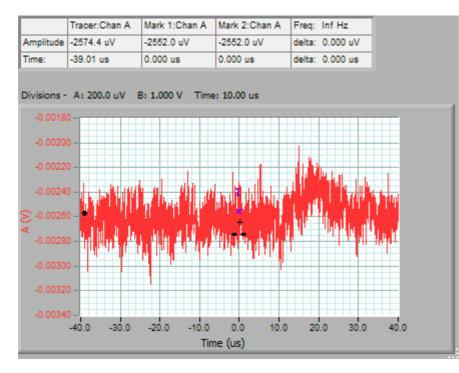
We can still see the outline of the signal, and the 200uV transient when the triggered LED is turned on. However the noise floor is 15dB worse than the previous graphs, and so the signal is much noisier.
