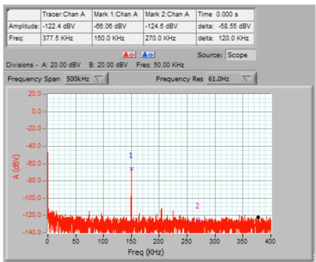
The 150 kHz signal amplitude is -66dBV. This is 10 \*\* (-66/20)= 501 uV.
