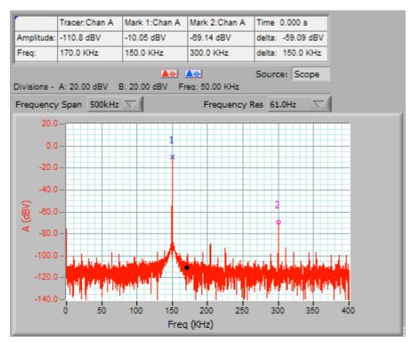
The noise floor is now about – 100 dBV, but there are intrusions – caused by the signal generator noise floor. The signal has been averaged 20 times.
