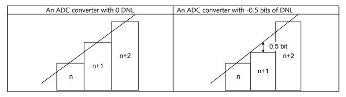
If we carry on increasing the period of the moving average filter, we will eventually expose the inherent nonlinearity of the ADC. Carrying on past this point yields no gain, as it is ADC defects we see, and not signal features.
