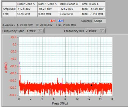
The 150 kHz signal can be seen highlighted by Marker 1. The amplitude is reported as –66.2 dBV, or 490 uV.
