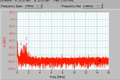
The entire Cleverscope acquisition unit was placed in an earthed Faraday cage (a metal box large enough to hold the unit and the antenna, with surrounding airspace space around the acquisition unit to allow internal radiation if it was occurring), and the following spectrum graph resulted:
