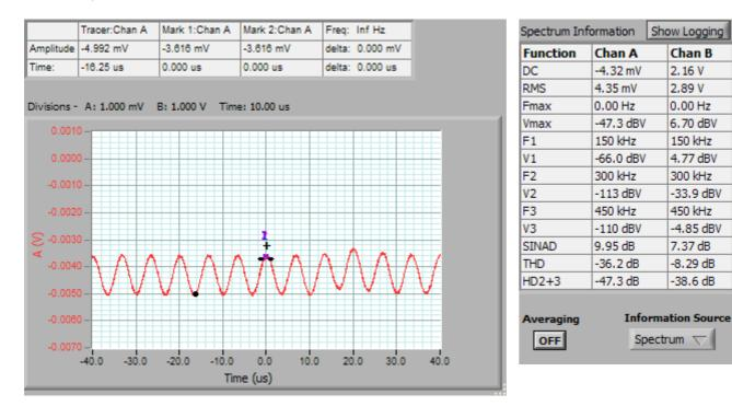
We used 20 averages. The information shows the amplitudes in the frequency domain, by using the spectrum graph as the information source.
