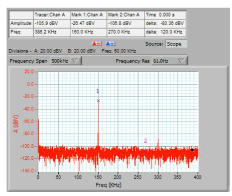
The spectrum graph shows-26.47 dBV (or 47.5 mV). We have about 74 dB headroom (so 5000x). This means we should be able to resolve 12 bits before being affected by noise. Next we use the same 30uV signal as before.
