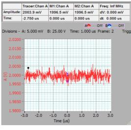
We have a dynamic range of  $\pm 2500$  mV, with a standard deviation of 1.9mV. This is 1 part in 2630, or a signal to noise ratio of 68.4 dB, equal to (68.4-1.76)/6.02 = 11.1 bits ENOB.
