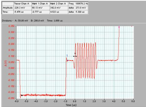
Normally the colour burst amplitudes are constant, as shown in this graph.
