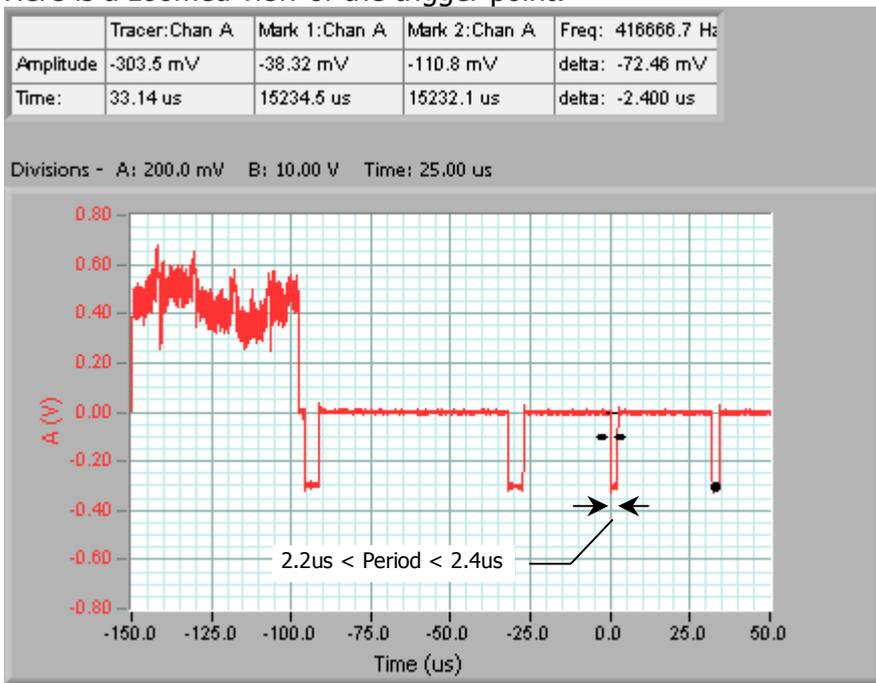
This method of using Trigger 2 (being Trigger 1 inverted) is useful for finding single pulses where the trigger level for both rising and falling edges is the same, and applies to the same source.
