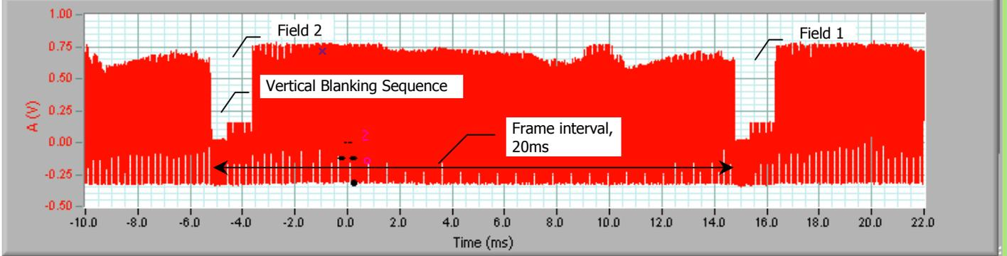
We can zoom in and see the vertical blanking sequence which establishes which field - Field 1 [first] or Field 2 [second] is being displayed.
