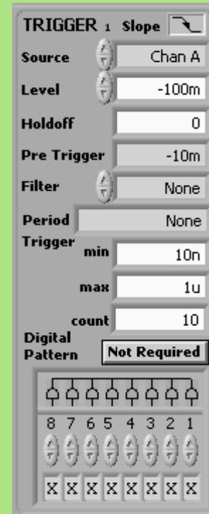
Here Chan A is the source, falling edge triggered at  $-100mV$ .
