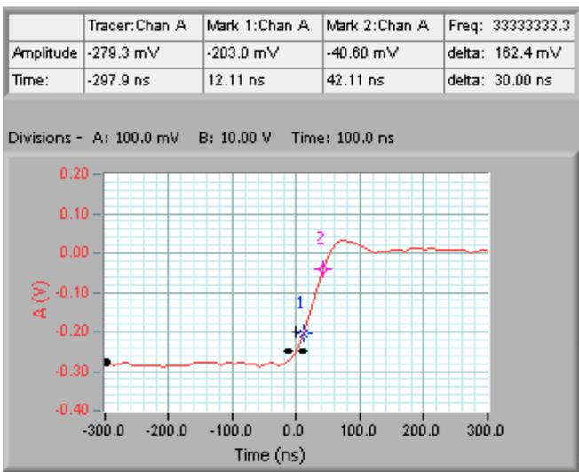
Next we set the min and max time values to 40ns and 1u, and found we captured no sync pulses. From this we can confirm that all sync pulses have a rise time of less than or equal to 30 ns.
