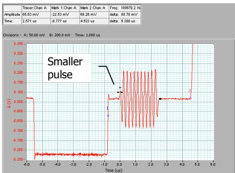
Notice that sometimes the first pulse is smaller than the others. We would like to trigger on this.
