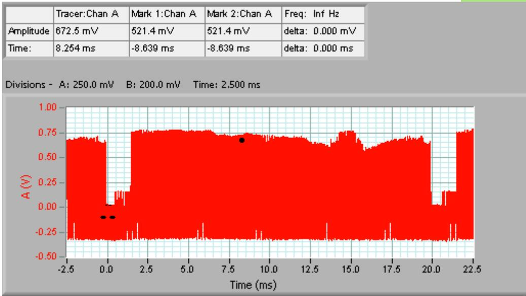
The trigger is the first pulse that meets the trigger specification.
