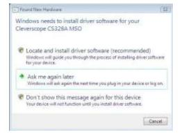
The PC should discover the USB connection and display 'Cleverscope CS328 MSO' or similar as in the dialog box. Click on "Locate and Install driver software" Wait after this for Windows to load the driver request dialog. (It might take some seconds as some installations go looking on the internet for a driver). Once the dialog comes up, choose to find the driver automatically.
